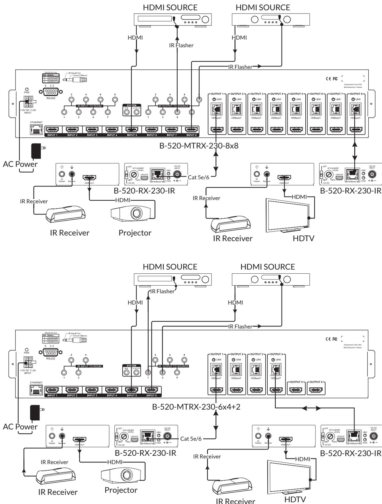
FIGURE 17: IR Passthrough
