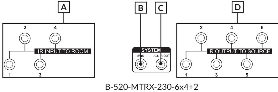
FIGURE 10: IR Connections
