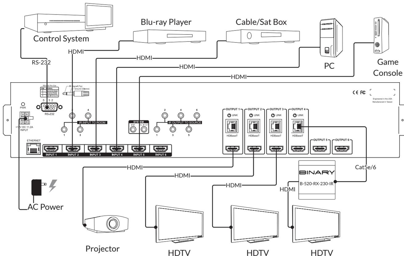
FIGURE 6: B-520-MTRX 6x4+2 Installation
