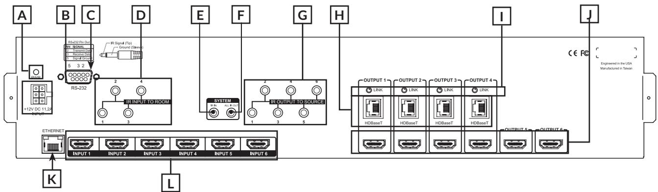
FIGURE 4: B-520-MTRX-230-6x4+2 Switcher Layout (Rear View)
