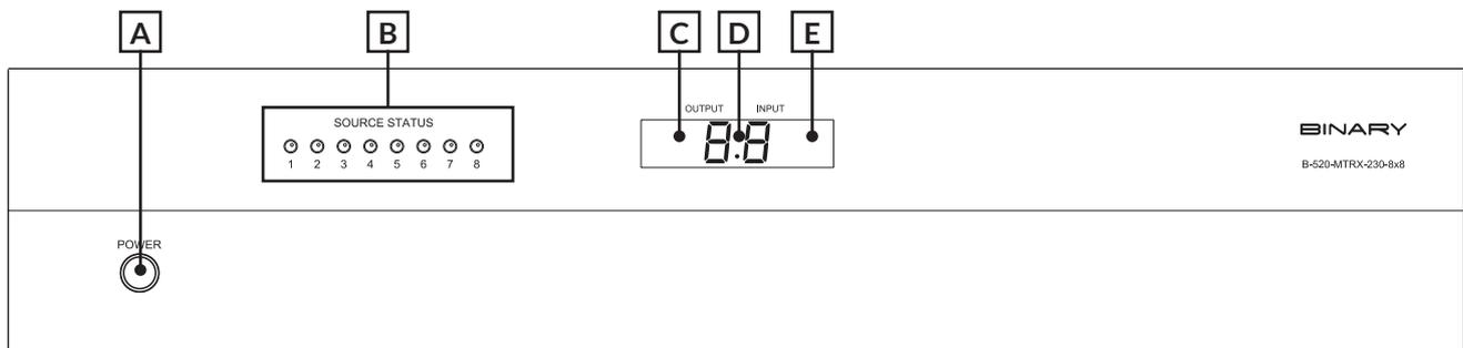
FIGURE 1: B-520-MTRX-230-8x8 Switcher Layout (Front View)
