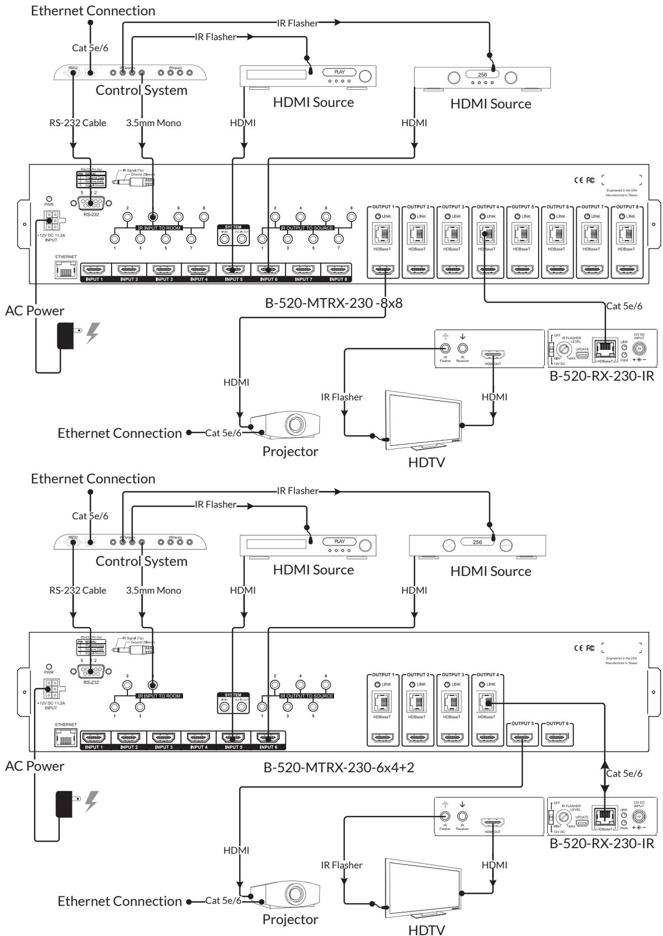
FIGURE 16: IR Passthrough Using Control System
