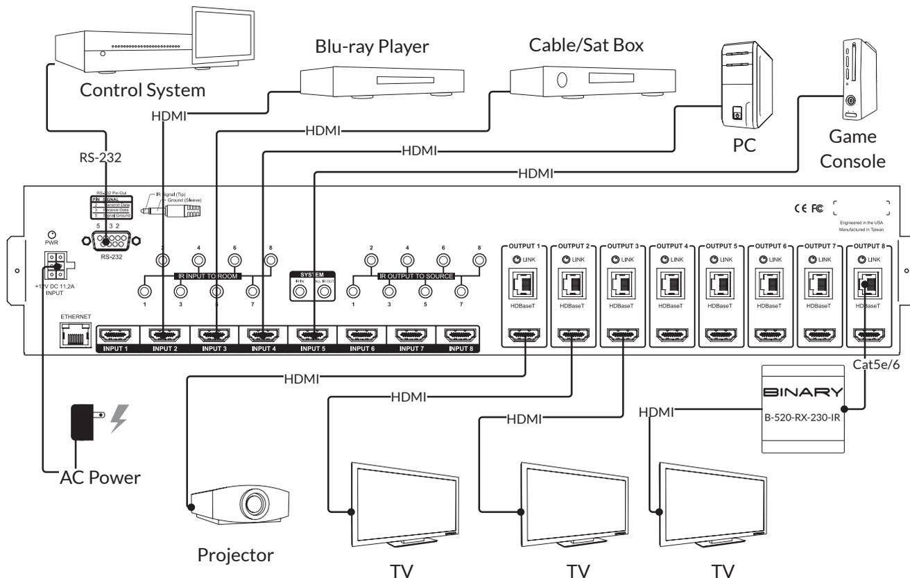
FIGURE 5: B-520-MTRX 8x8 Installation
