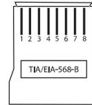
FIGURE 7: RJ45 Pinout Configuration
