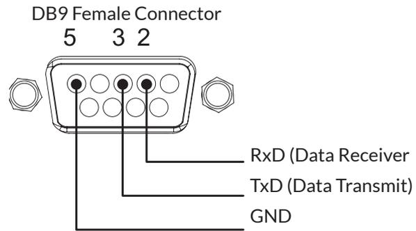
FIGURE 9: RS-232 (DB9) Pin Configurations
